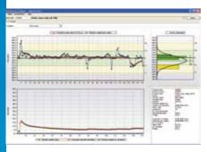
Dashboard style monitoring of variables with information displayed alphanumerically and graphically for important values such as production mean values, random sample mean values or individual values of spot-checks.
