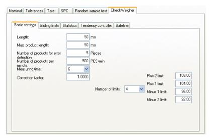
Clear and comprehensive configuration of the checkweigher in FreeWeigh.Net®
